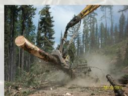
FIGURE 3: Dangle-head processor.
